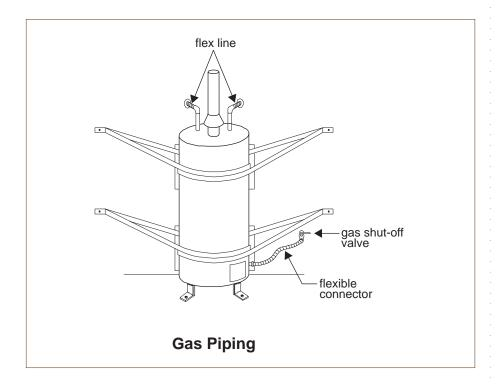
Gas piping may break, causing gas leaks that can harm nearby occupants, or starting a fire.
