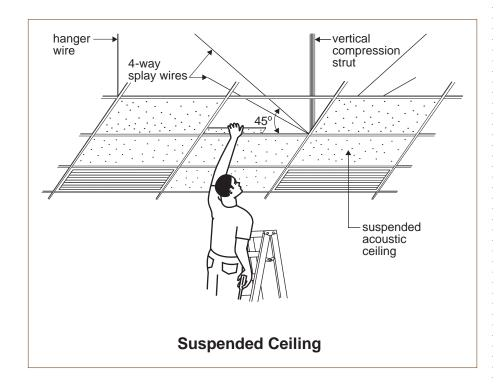
Unsecured suspended ceiling may fall, striking occupants below or blocking exit ways for evacuation during an emergency.
