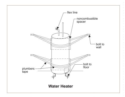
Unsecured plumbing equipment such as a water heater may slide or fall,
