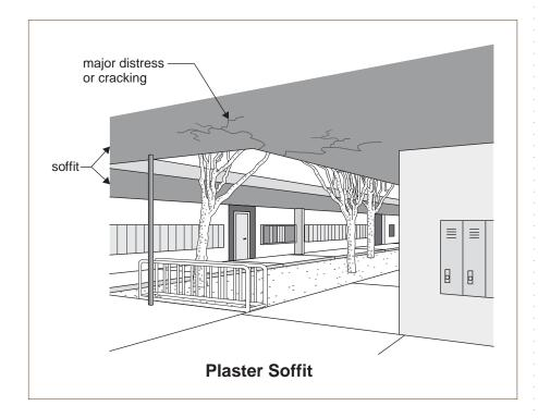
Deteriorated plaster may collapse, striking occupants below or blocking hallways and exit ways during an emergency.
