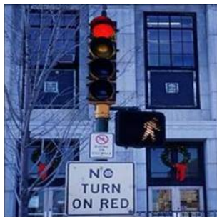
Restricting right turns on a red light can help reduce conflicts between pedestrians and drivers.
