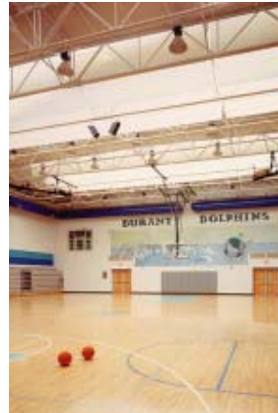
Monitors provide diffuse light into gymnasiums. NREL/PIX 11338
