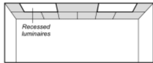
Recessed luminaires are direct general light source.
