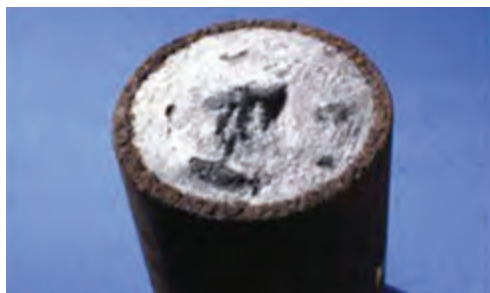
Figure 9.2.8. Boiler tube – scale deposit
