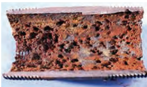
Figure 9.2.12. Condensate pipe – oxygen pitting
