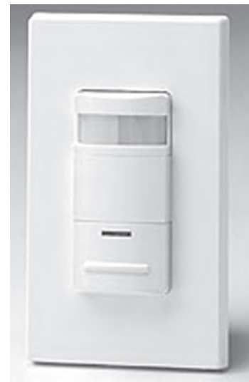
Figure 9.12.2. Wall-box occupancy sensor uses hidden internal dip-switches to set manual-on, auto-off.
