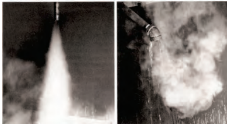
Figure 9.3.7. Live steam (left) versus flash steam (right)
