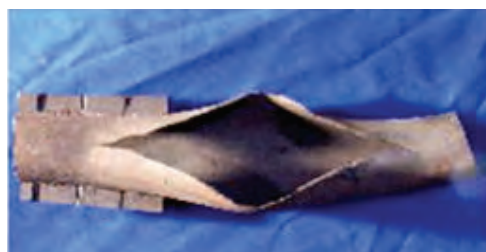
Figure 9.2.11. Boiler tube – failure (rupture)
