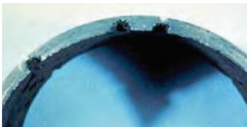
Figure 9.2.10. Feed-water pipe – oxygen pitting
