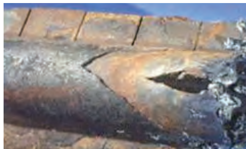
Figure 9.2.9. Boiler tube – failure (rupture)
