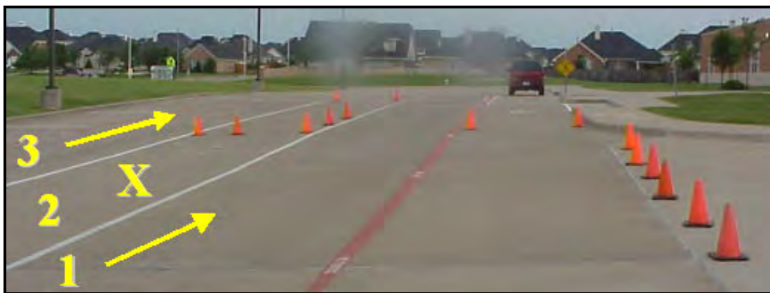
Figure 28. Placement of Traffic Cones to Create a Dual-Lane Queue.
