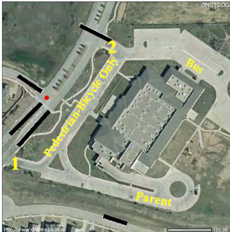
Figure 9. School with Good Physical Separation of Basic Modes of Traffic Pattern (14).
